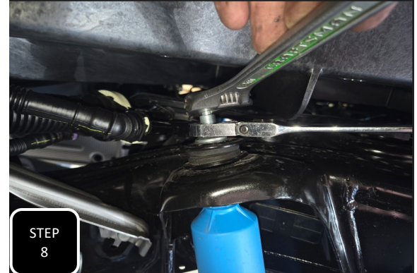
Step 8 Re-attach both shocks and tighten. NOTE: IF THE REAR COILS ARE TOUGH TO COMPRESS AND THE TRUCK STARTS TO LIFT OFF OF THE CAR LIFT. LOWERING THE TRUCK TO THE GROUND ALLOWS THE WEIGHT OF THE TRUCK TO COMPRESS THE SPRINGS AND MAKE THIS STEP EASIER.
