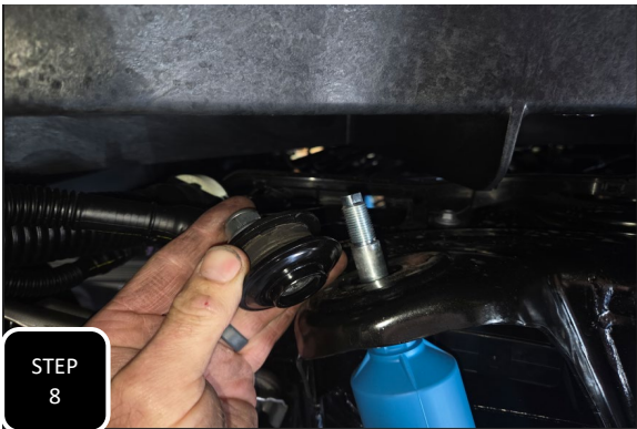
Step 8 Re-attach both shocks and tighten. NOTE: IF THE REAR COILS ARE TOUGH TO COMPRESS AND THE TRUCK STARTS TO LIFT OFF OF THE CAR LIFT. LOWERING THE TRUCK TO THE GROUND ALLOWS THE WEIGHT OF THE TRUCK TO COMPRESS THE SPRINGS AND MAKE THIS STEP EASIER.
