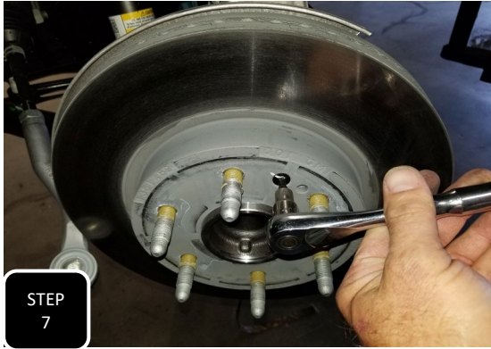
Step 7 Unbolt the rotor retainer bolt and remove the rotor.
